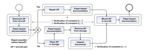
Fig. 1. Simplified model of a maintenance process from the aviation industry
