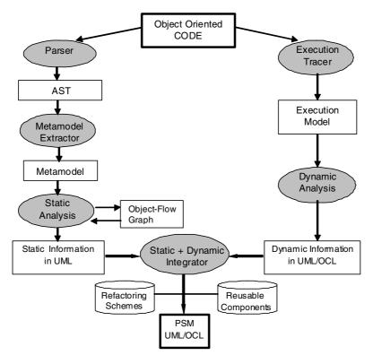
**Fig. 2.** Reverse engineering at model level: static and dynamic analysis
