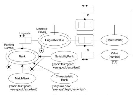
Fig. 7. Object-Role Modeling (ORM) model of the fuzzy match functions.
