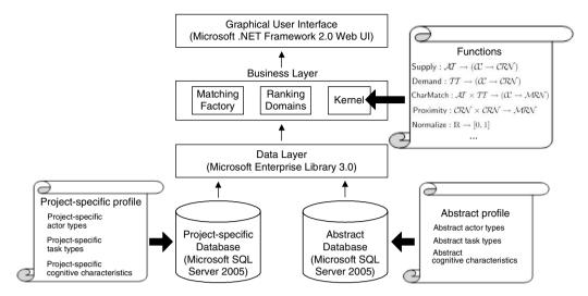
Fig. 8. Cognitive matchmaker system architecture.
