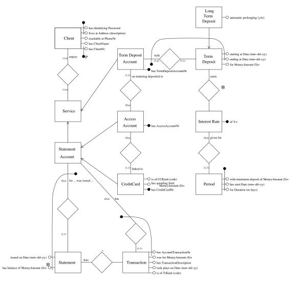
Figure 4.19: Complete ER diagram of the Bank domain
