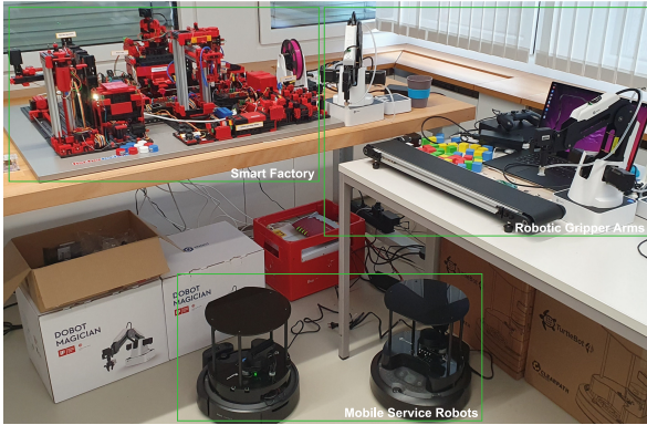
Fig. 5. Extended smart manufacturing setup with new CPS.
