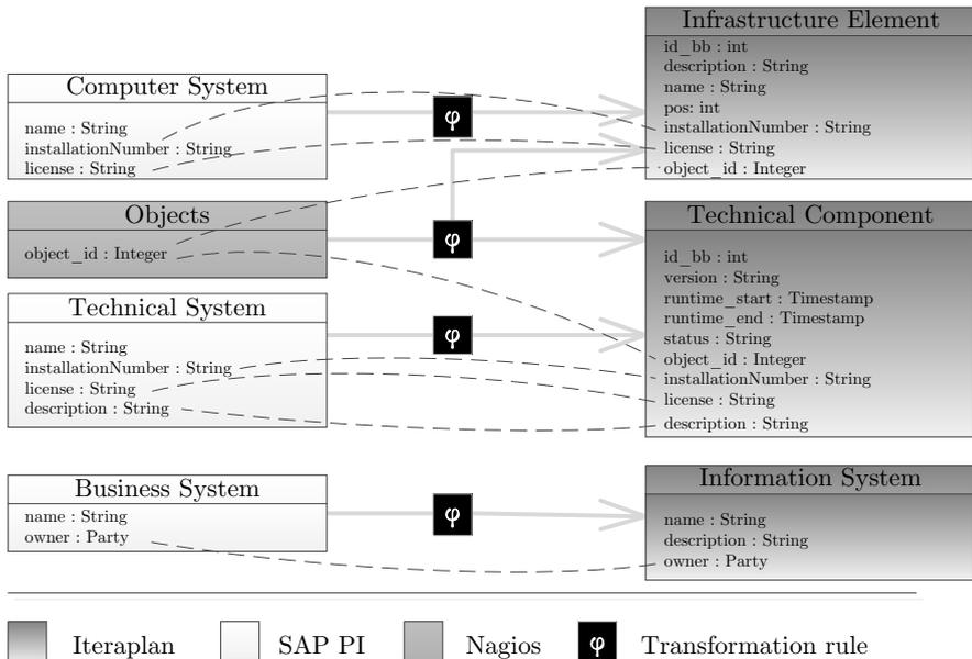
Fig. 6. Data model mapping of SAP PI and Nagios to Iteraplan
