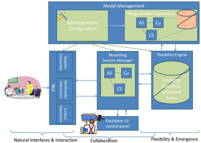
Fig. 2. Natural Enterprise Modelling Infrastructure - Conceptual Architecture
