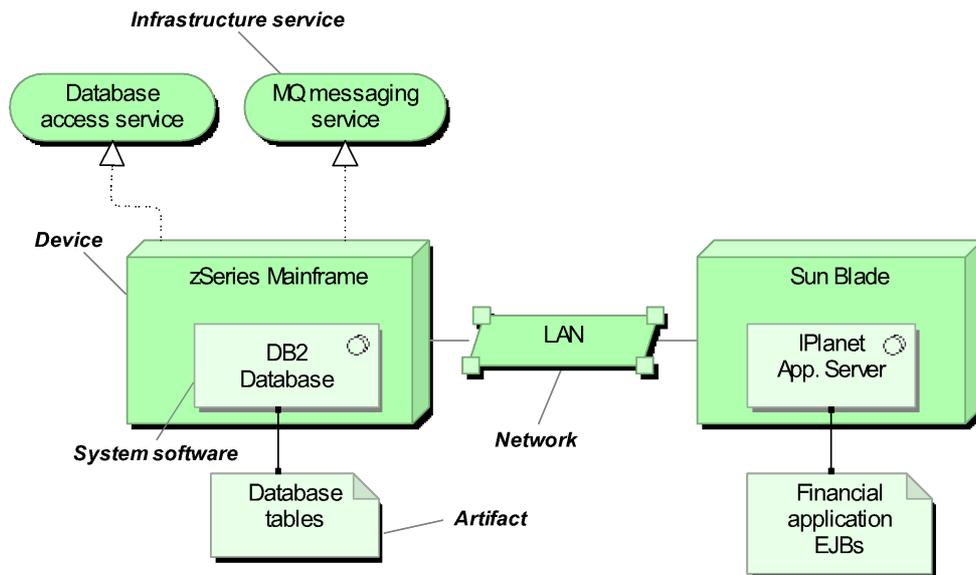
Figure 17. Technology layer example model
